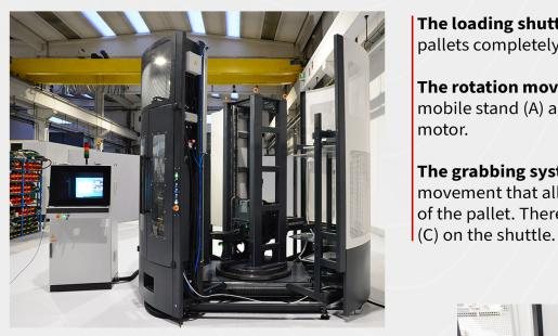
Flexible Pallet Tower FTP is composed of a transport shuttle equipped with an elevator and a series of positions on a two-storey warehouse.
