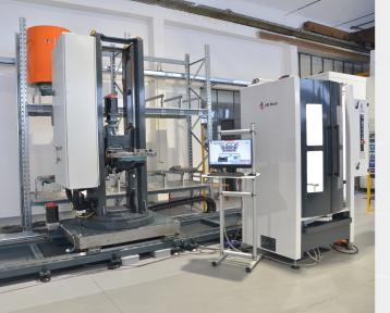
**Flexible Pallet Linear** is composed of a transport shuttle equipped with an elevator and a series of positions on a two-storey warehouse.
